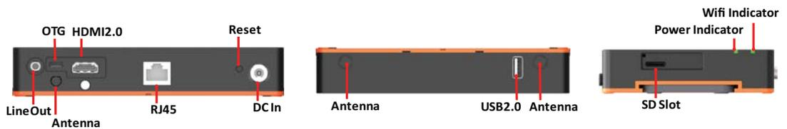
Figure 2.4 IO Layout of USM-110 Delight Version
