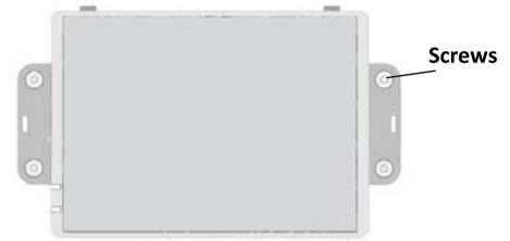
Screw specs: length >15 mm; diameter <4 mm
